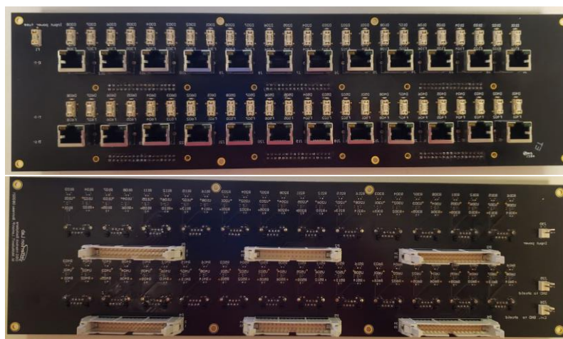
Front and back side of fully populated Backplane PCB
